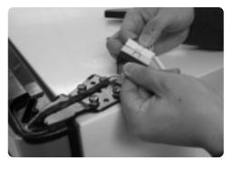
3. With the 10 inch wrench, remove the four bolts that hold the top of the refrigerator.
